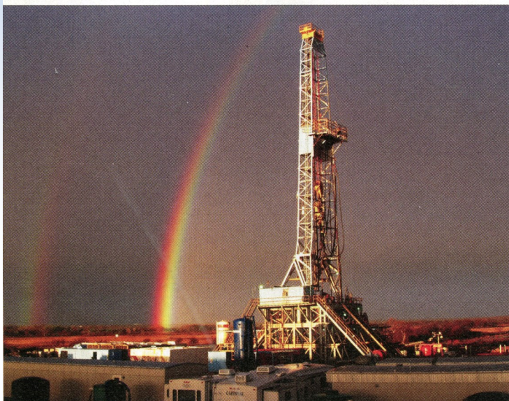
Top: Latshaw Drilling's Rig 19 features hydraulic "walking feet" (in yellow) on the substructure to allow the rig to walk for multiwell pad drilling. Bottom: Latshaw's Rig 8, a National 1320-UE rig, is operating in the Permian for Tall City Exploration. The 2,000-hp SCR rig also features a walking system.
