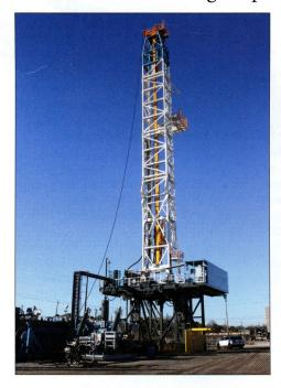
Two new rigs from Latshaw Drilling began operations in December in the Permian Basin. The first is Rig #42 (pictured), a National Oilwell Varco (NOV) Ideal 1,500-hp AC rig with a Varco TDS-11, 500-ton AC top drive unit. It features two NOV 12-P-160 mud pumps with 7,500-psi fluid ends and a BOP handling system. The rig is outfitted with the first walking system that NOV has installed on an Ideal rig.
