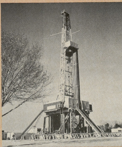
Front Cover: Latshaw Drilling's Rig No. 2 is pictured drilling a 15,000-ft exploratory well for Arco in Lavaca County, TX. The photograph of the 25,000-ft capacity diesel-electric SCR drilling unit was taken by Trent B. Latshaw, company president. The rig has since moved on to another well for Arco, a 17,000-ft exploratory well in Bee County, TX.
